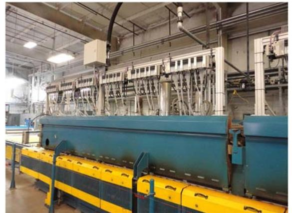
efficient Mroczek furnace, only used when demand increases. Lockheed Martin Energy's Heavy Industry Energy Efficiency Program (HIEEP) performed a site audit to identify potential energy savings, and found opportunities through automating the glass seaming operation.
